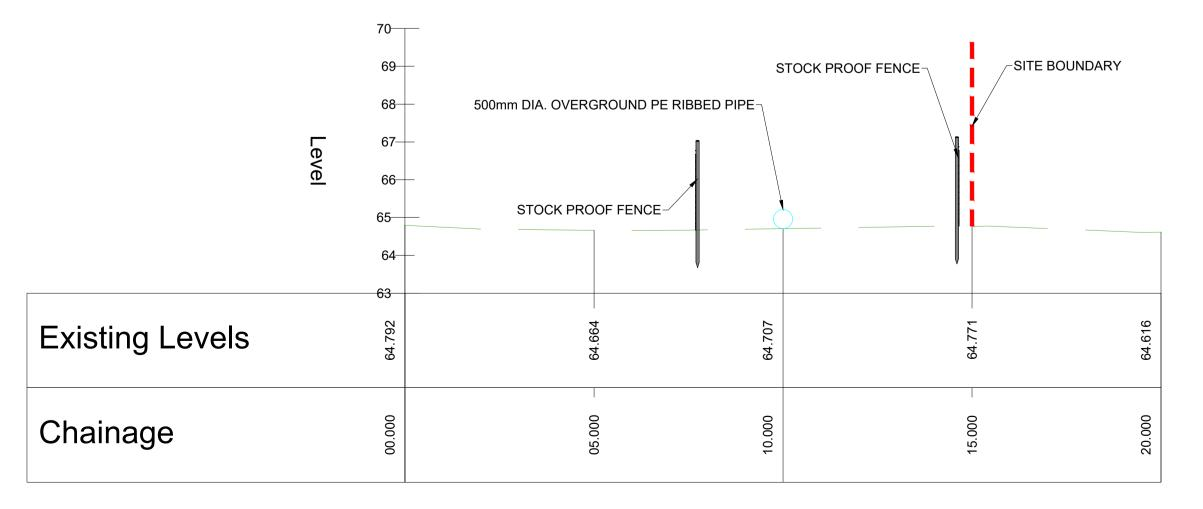
SECTION D-TYPICAL SECTION THROUGH PIPELINE WITH 500MM DIA. HDPE RIGID PIPE
